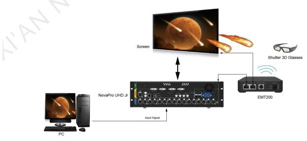
Figure 3-30 3D solution architecture
